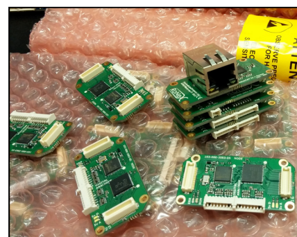
Figure 7: The new RoNeX boards stacked together.
